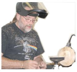
With wood being so expensive, Mark showed us how to make some very effective bowls and vases from 1" thick Oak board. A 1" x 8" board was mounted on a screw chuck. After turning it to round, Mark used a 1/4" bowl gouge to create a saucer shape on the bottom. He then ebonised the surface with a Mapp gas blow torch (extraction MUST be off at this point). A water spray doused any embers, followed by burnish-
