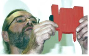
When he was satisfied with the flowing shape, Mark stopped the lathe and cut the three legs by hand, using a Japanese trim saw.
