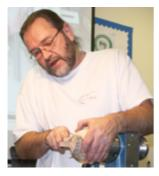
Mark's project was a three-legged vessel in Oak. Mounting the blank between a steb drive centre and a ring centre, he used a spindle roughing gouge to true up the piece. This was followed by a long grind bowl gouge to rough out the shape. Mark cut a parallel chucking spigot at the tailstock end and reduced the diameter of the section where the legs would appear. The blank was then mounted in a chuck. Mark squared off the end with a normal grind gouge and made a small
