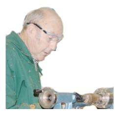
Ron started with a Yew blank, 3" square and 8" long. This was enough for an apple and a pear. After rounding over the top of the pear, Ron drilled a hole in the end for the stalk. Ron then used a spindle gouge to shape the pear, followed by sanding, sealing, buffing and parting off.
