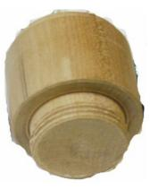
the box in the chuck, Phil marked the required thread diameter and cut it slightly oversize. He cut another recess at the end of the threaded portion and cut a chamfer as before. Using the external thread chaser, Phil cut the
