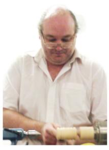
Rob's project was a gavel in Yew. With the blank held in a chuck, Rob used a spindle roughing gouge to turn it round, removing all of the bark in the process. He then squared off the end with a skew chisel and parted off the waste at the chuck end. After mounting the spigot in the chuck, Rob used a gouge to cut the shape of the gavel head. Rob sanded and waxed the piece before buffing it with a real chamois leather. He then parted off using a narrow parting tool.
