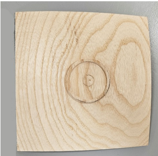
The finished thin platter with very shallow chucking recess.
