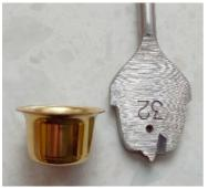
"spade" drill bit that I have ground to the shape of a candle cup. Shape the "apple" top with a spindle gouge.
