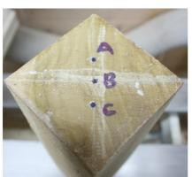
square, mark the centres at each end using the corner to corner method. Using one of the corner to corner lines, mark another two offset centres (A & C) 16mm either side of the true centre. Repeat this at the other end making sure the same diagonal and orientation is used. Then mount the blank between the true centers (B), turn it to 65mm round and add a chucking spigot at the tailstock end. Do not lose the centre markings.
