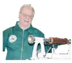
Stan's project for the evening was an open bines vase in mahogany (from an old newel post). Mounting the blank between steb centres, Stan cut a chucking spigot with a parting tool and created a dovetail using a skew chisel. He then mounted in the chuck and brought up the tail stock for support. Stan turned the blank to a cylinder and squared off the end. He then turned a cove down to the
