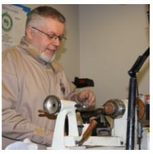
Frans started the evening by turning a pendant out of burr oak. To do this, he used a home made offset glue chuck. Using a very simple but effective construction, the jig sat in the gap between the chuck jaws. Simply
