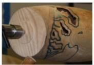
the wood is completely dry, Frans used a Dremel rotary tool (with foot control) and carbide burrs to carve out the shapes. The cut-off top was replaced to support the piece during carving.
