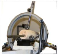
To support the piece whilst hollowing, Frans used a home-made 3 wheel steady. This uses soft skateboard wheels and the arms are not at 120° i.e. not equally spaced so as to avoid harmonic resonance. The jig is also useful to support segmented work. Frans started his hollowing by drilling a large hole down the centre. He then demonstrated his hollowing jig. This consists of a hollowing cutter mounted on an articulated arm. The arm
