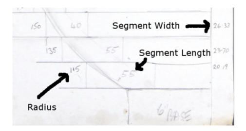
Part of the plan for a vase. Drawn to scale so that measurements may be taken directly from the drawing rather than calculations. Lengths & widths then added from the solid or open segment tables.
