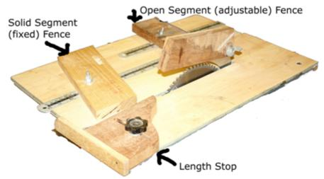
John's table saw jig for cutting segments. The fixed angle fence for solid segments is shown. The adjustable angle fence for open segment work is also on the table.
