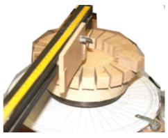
radius that was taken from the drawing. Using ordinary PVA glue, a segment is placed against the stop and held for a few moments while the glue takes hold. The plate is rotated to the next mark and the next piece placed. This is repeated until the layer is complete. The arm is raised and the next later placed. After a few layers have been placed, John will remove the part-vase, still held on the faceplate, and turn the inside. The top (unsupported) row is not turned.
