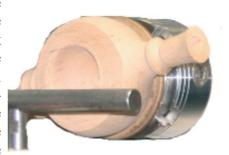
entrance hole needs to have a square shoulder to take the bung that will be turned later. After sanding, the piece is reversed onto the chuck jaws and the other side is hollowed. Paul uses Rustins Plastic Coating to seal the inside.
