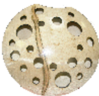
Version 1: Different sized holes using a forstner bit.
