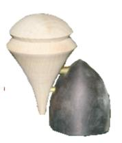
a smooth curve down to a narrow rounded point. He made several refining cuts to the curve, to ensure it matched the curve on the base. Robin hollowed the inside and cut a small shoulder on which, the lid would rest. He then sanded, sealed and finished it with a clear lacquer.
