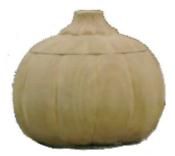
ends and shaped the head round at both ends, with the widest part about 3/4" to 1" from the top, and tapered to both ends. After drilling a 25mm hold down the centre from both ends, Emma decorated the top. She then turned the handle, making it protrude 10mm from the head and only long enough for the user's hand size to the wrist bone. Any longer and the mallet can't be used properly. She also cut a thumb notch so that, without looking, it is always oriented to hit with the end grain.
