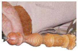
mica to burn in the lines. He then sanded 120 grit to 400 grit before sealing and waxing as before. After aligning the grain direction, the spigots were inserted into the holes in the plates. The top spigot only needed one spigot, with a ball on the other end to act as a handle.
